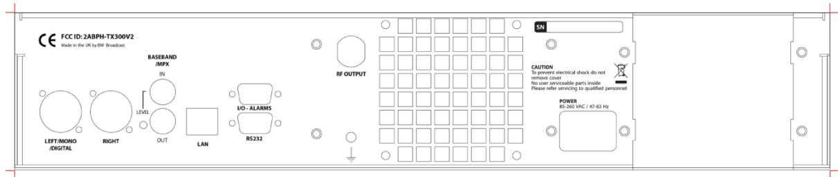
There are two options how the label will be affixed to the unit. For standard production the label will be a part of non removable rear panel silk screen. For labelling the existing units a permanent sticker will be used.
