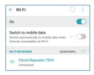
3. Once connected, open an internet browser on your smartphone or tablet and enter the address 10.10.10.254. The Ferret Repeater configuration page will open up.
