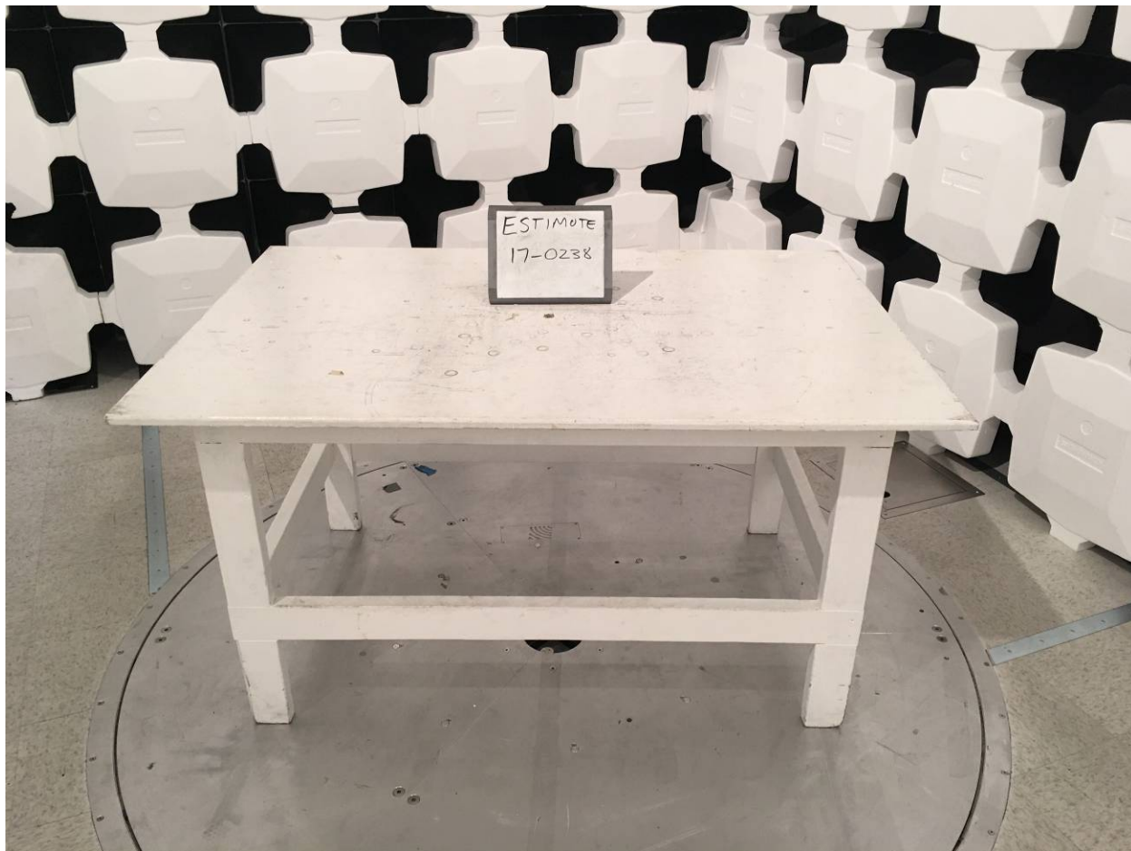
Figure 6. Unintentional Radiated Emissions Test Configuration Setup
