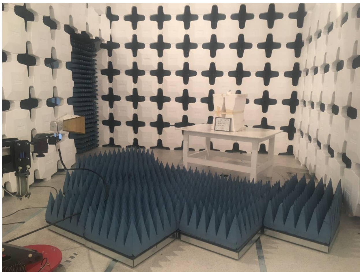
Figure 2. Intentional Radiated Emissions Test Setup, Above 1GHz
