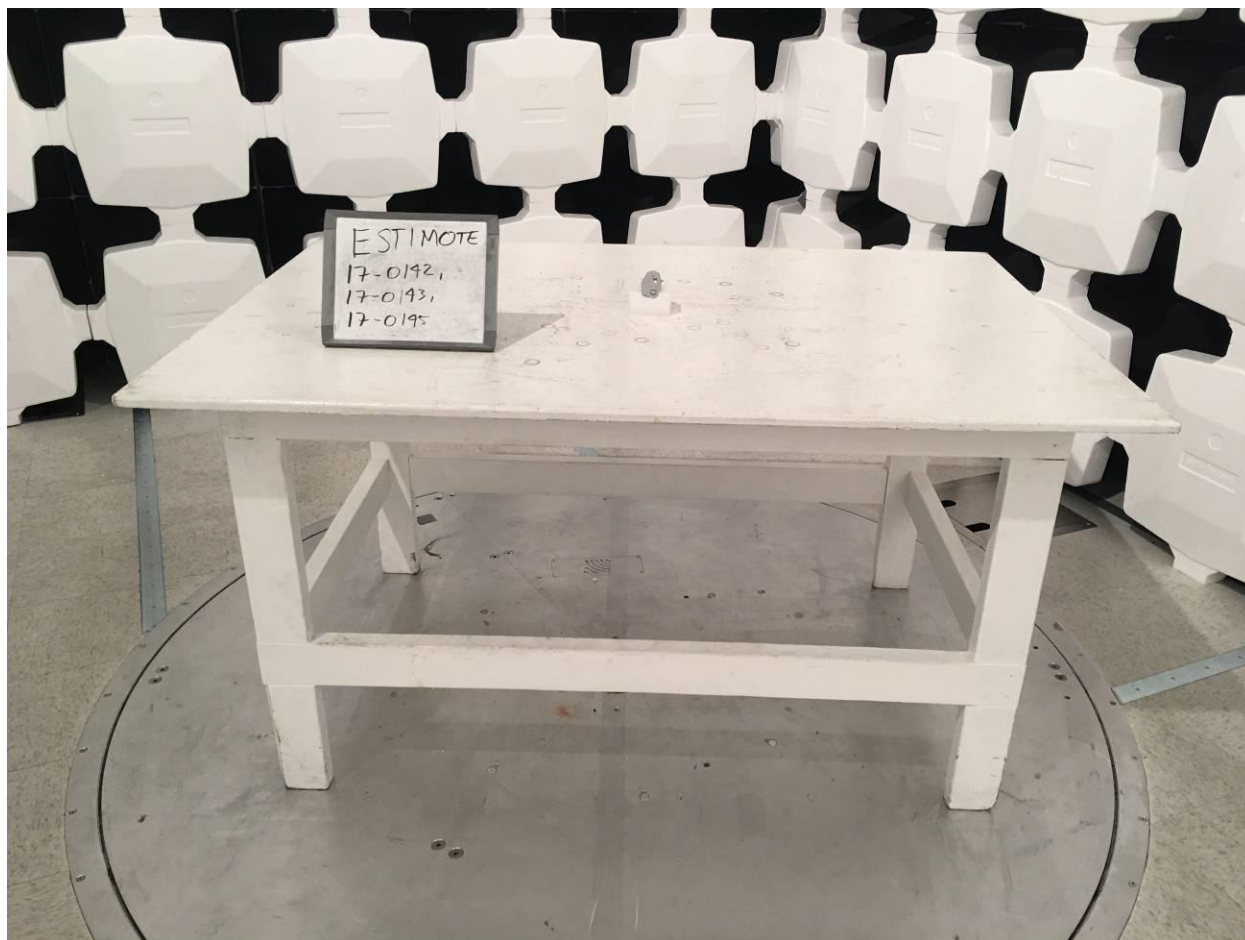
Figure 9. Unintentional Radiated Emission Test Setup, Front
