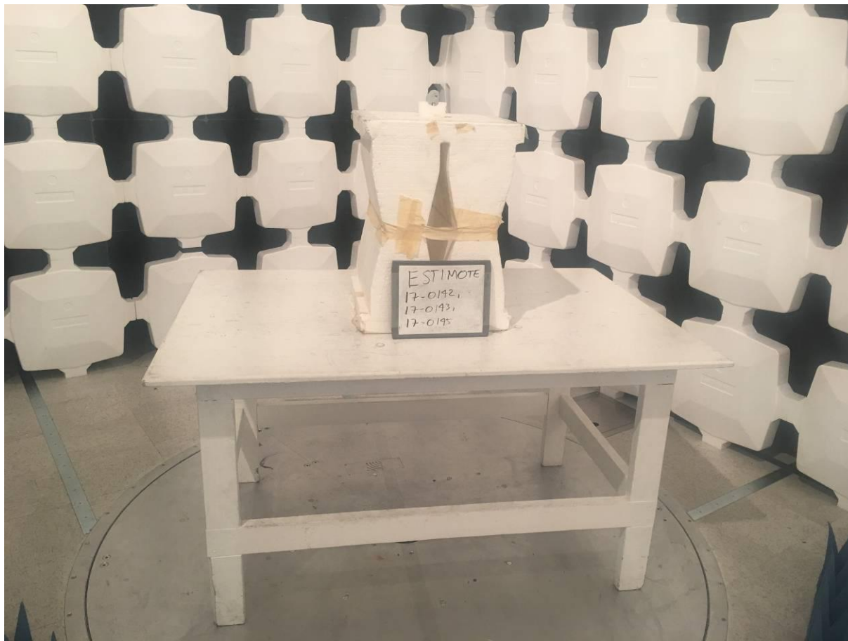
Figure 1. Intentional Radiated Emissions Test Setup (Worst Case Position)
