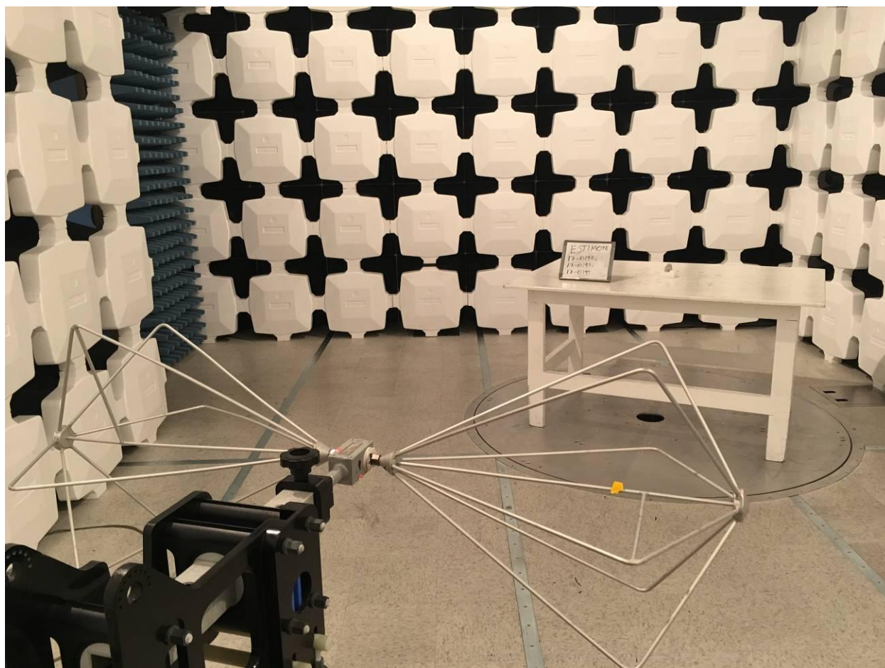
Figure 6. Radiated Emissions Test Setup, 30 MHz to 200 MHz (For Both Intentional and Unintentional Emissions)
