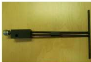
Figure 1 – MVG COMOSAR Validation Dipole
