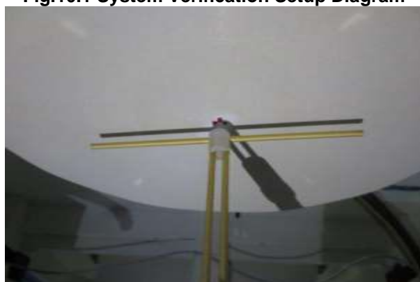
Fig.10.2 Photo of Dipole setup
