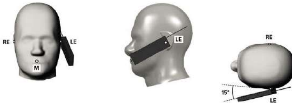
Fig.11.4 Illustration for Tilted Position
