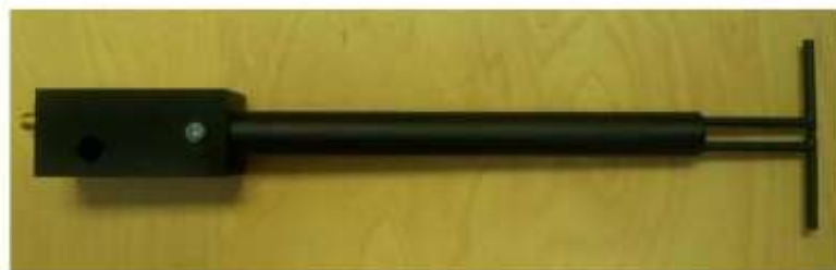
Figure 1 – MVG COMOSAR Validation Dipole
