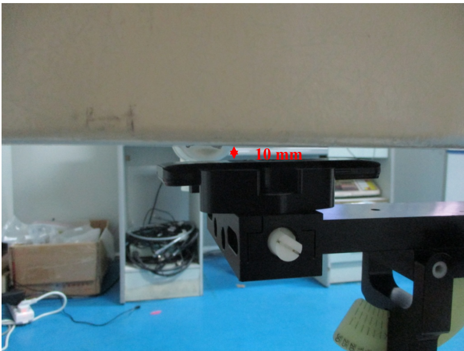
Body (Worn) Back Setup Photo(10mm)
