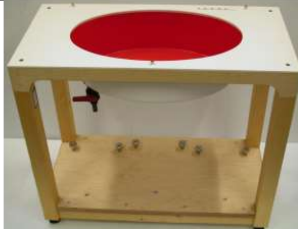
Fig.8.8 Photo of ELI4 Phantom
