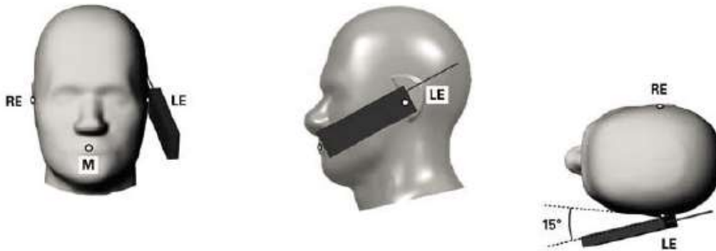
Fig.11.4 Illustration for Tilted Position
