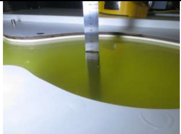
Fig. 9.2 Photo of Liquid Height for Body SAR (850MHz) (depth>15cm)
