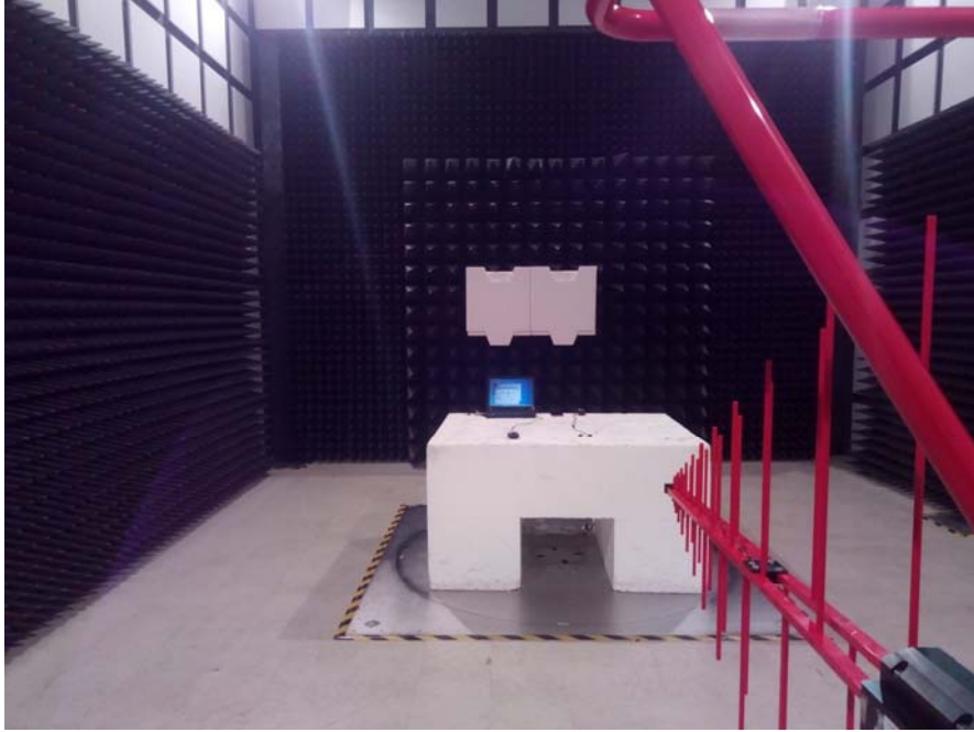
Radiated Emissions – Front View (Below 1 GHz)
