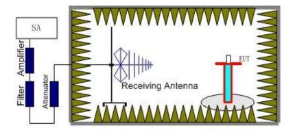
Radiated emissions measurements were made only at the upper, middle, and lower carrier frequencies of all modes. It was decided that measurements at these three carrier frequencies would be sufficient to demonstrate compliance with emissions limits because it was seen that all the significant spurs occur well outside the band and no radiation was seen from a carrier in one block of any band into any of the other blocks.
