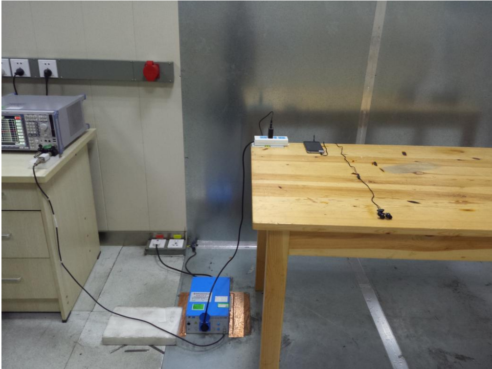
FCC RADIATED EMISSION TEST SETUP
