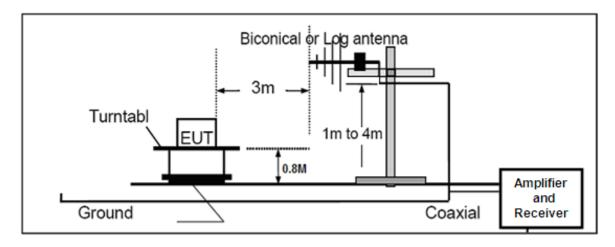
RADIATED EMISSION TEST SETUP ABOVE 1000MHz
