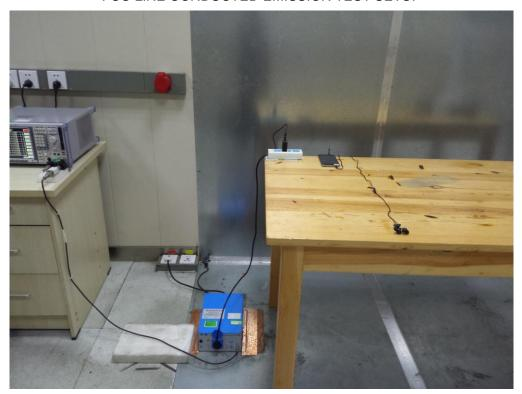
FCC RADIATED EMISSION TEST SETUP
