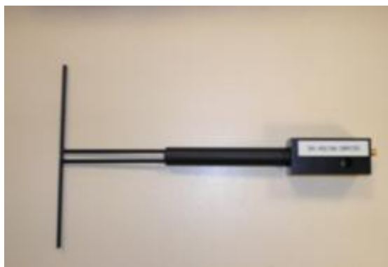
Figure 1 – Satimo COMOSAR Validation Dipole
