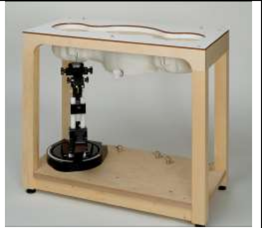
Fig. 8.7 Photo of SAM Twin Phantom
