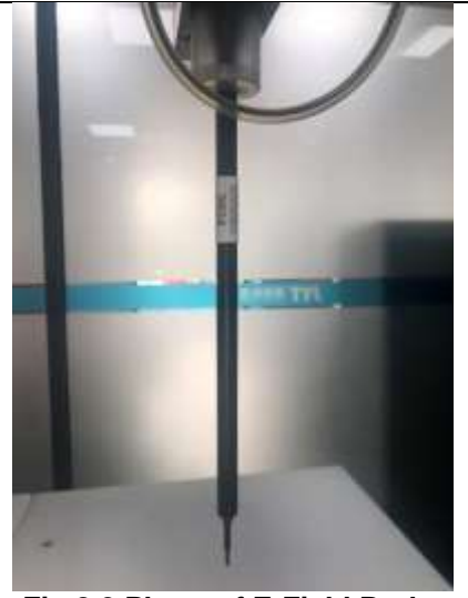
Fig.8.2 Photo of E-Field Probe
