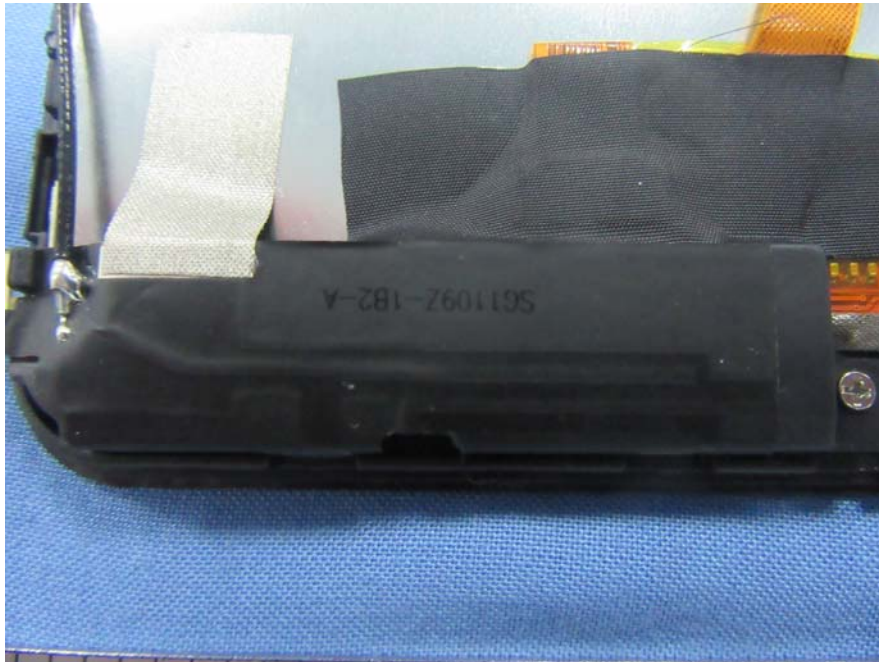
EUT – GSM&WCDMA Antenna View
