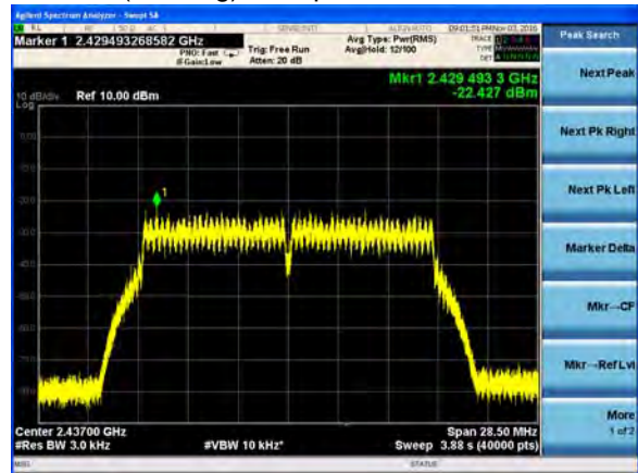
(802.11g) PSD plot on channel 6
