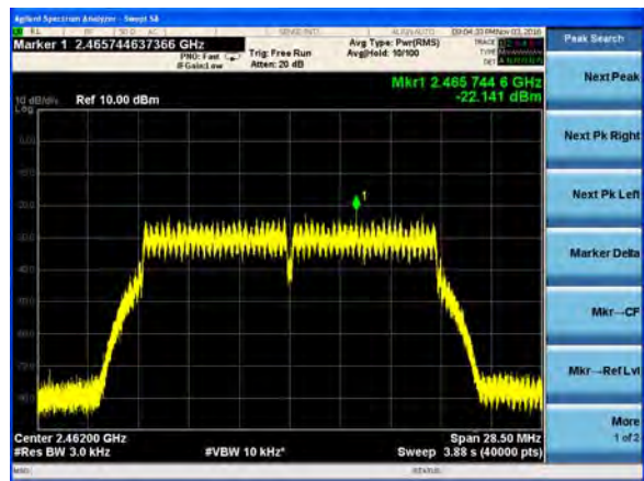
(802.11g) PSD plot on channel 11
