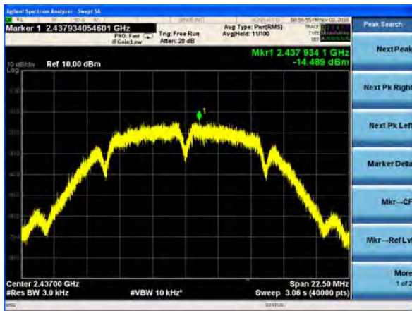
(802.11b) PSD plot on channel 11
