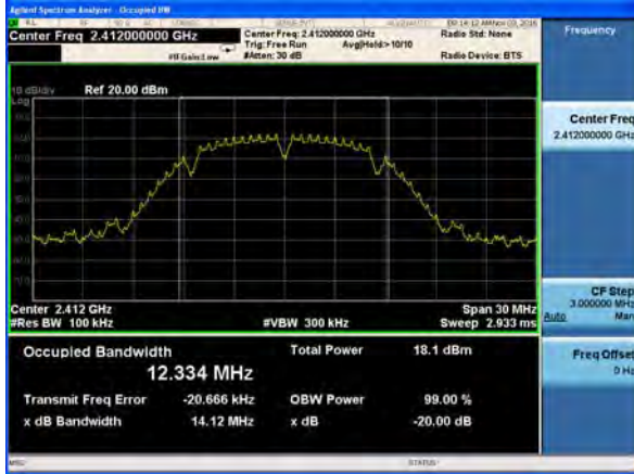
(802.11b) -20dB Bandwidth plot on channel 1
