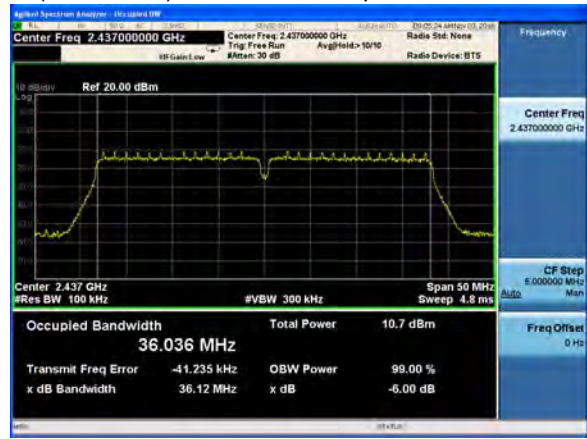
(802.11n40) 6dB Bandwidth plot on channel 6
