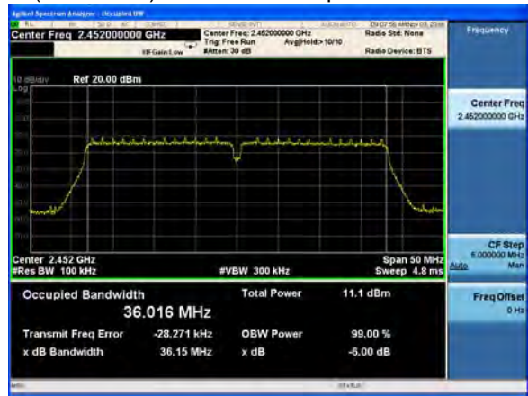
(802.11n40) 6dB Bandwidth plot on channel 9
