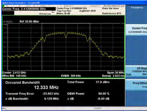
(802.11b) 6dB Bandwidth plot on channel 1
