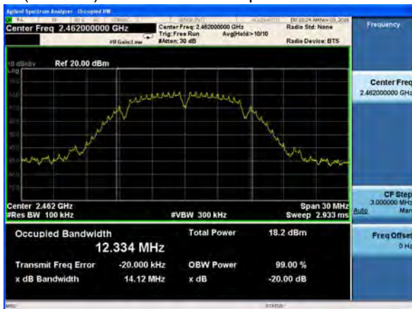
(802.11b) -20dB Bandwidth plot on channel 11
