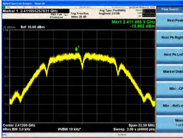
(802.11b) PSD plot on channel 6
