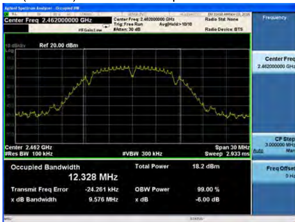
(802.11b) 6dB Bandwidth plot on channel 11
