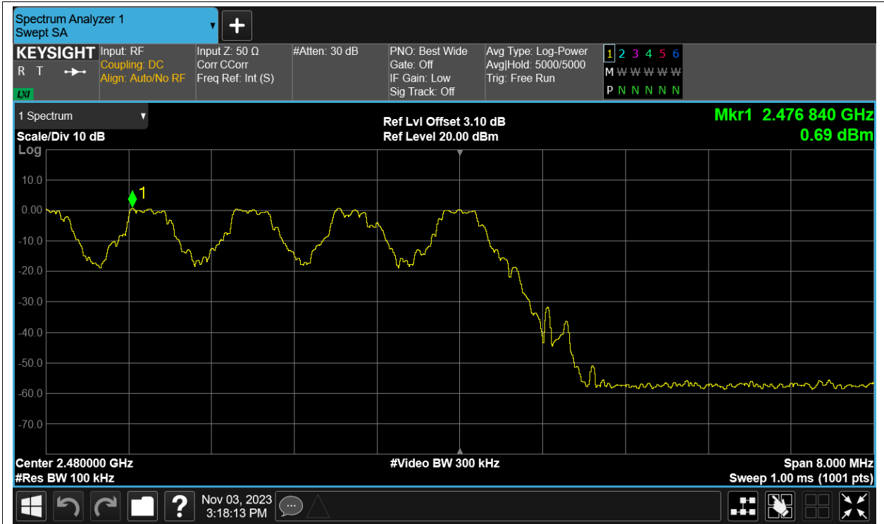
Band Edge(Hopping) NVNT 1-DH1 2480MHz Ant1 Hopping Emission
