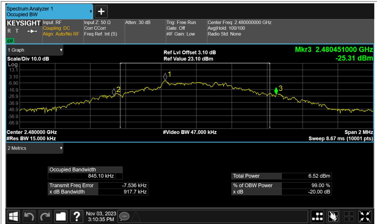
-20dB Bandwidth NVNT 2-DH1 2402MHz Ant1
