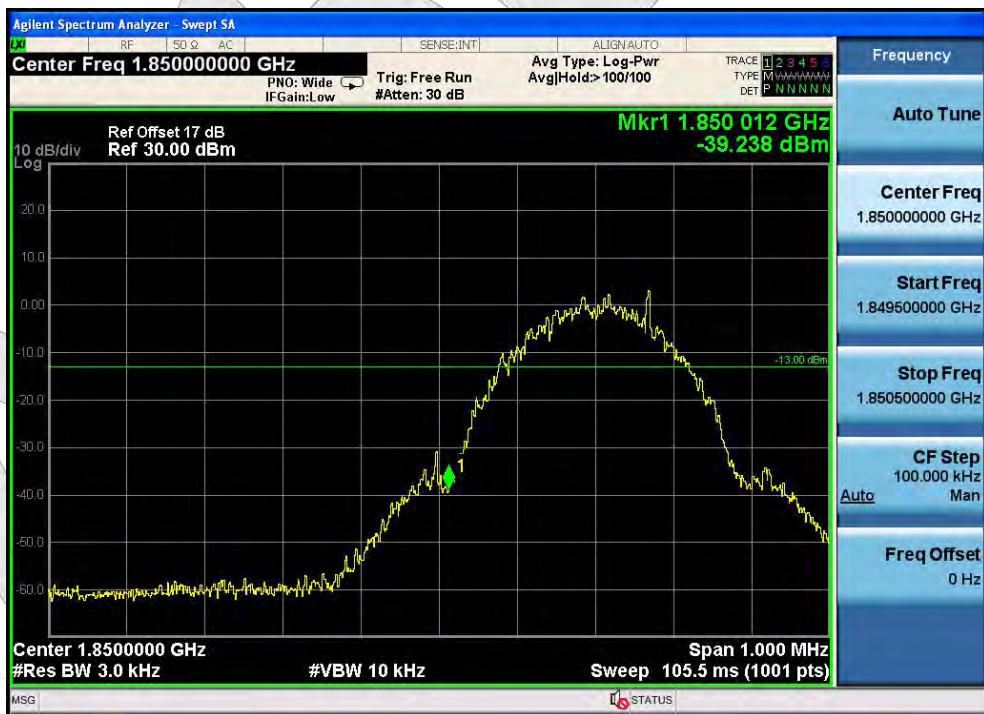
Test Mode: GPRS 1900 - Low Channel
