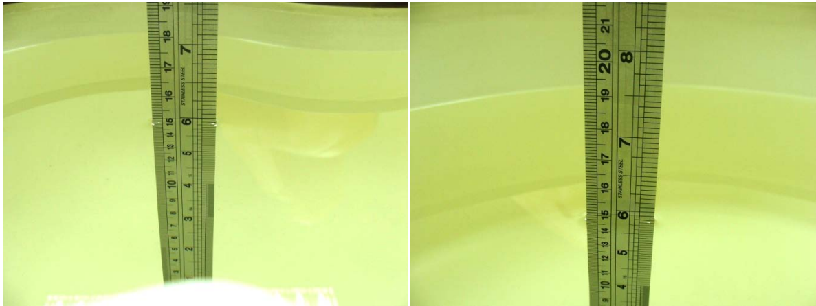
Photo of Liquid Height for Head SAR
