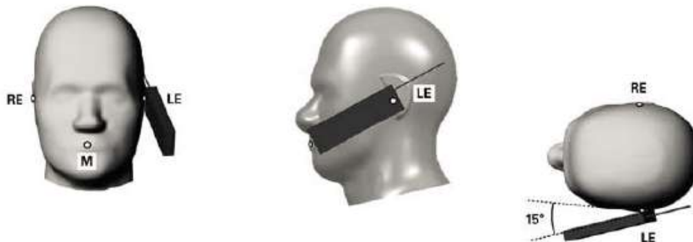
Fig.11.4 Illustration for Tilted Position
