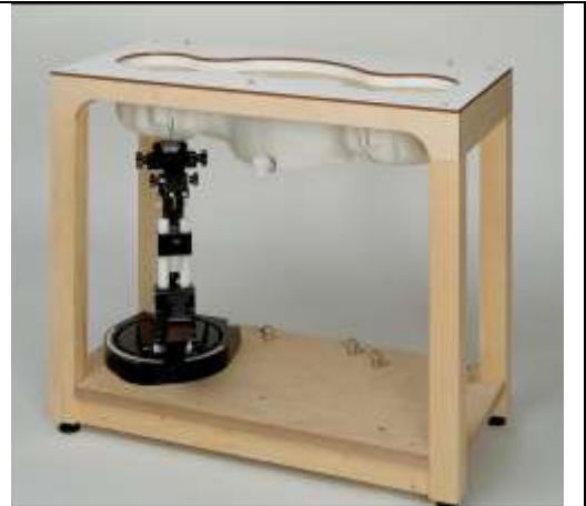
Fig. 8.7 Photo of SAM Twin Phantom
