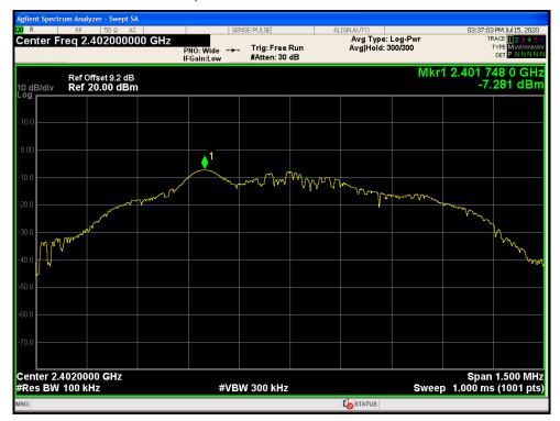
Tx. Spurious NVNT BLE 2402MHz Ant1 Emission
