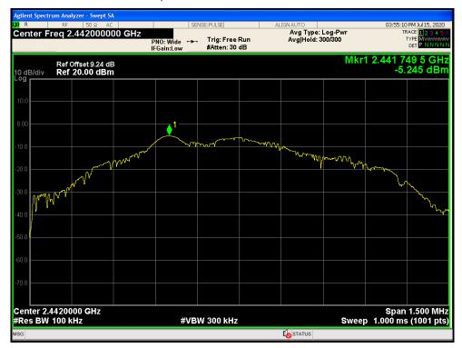
Tx. Spurious NVNT BLE 2442MHz Ant1 Emission
