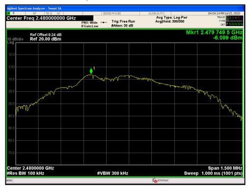
Tx. Spurious NVNT BLE 2480MHz Ant1 Emission
