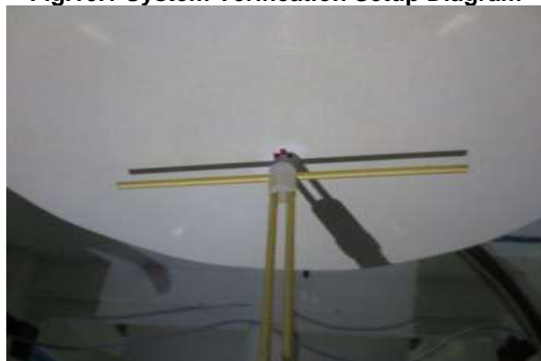
Fig.10.2 Photo of Dipole setup
