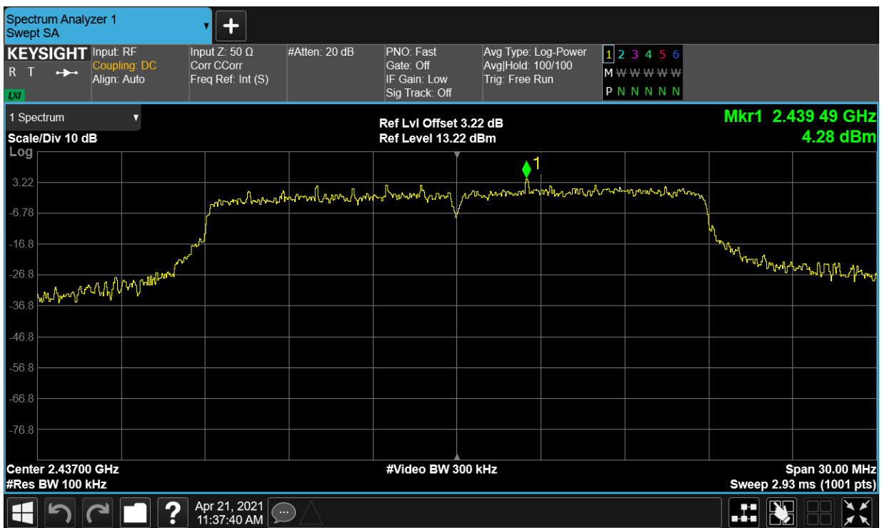
Tx. Spurious NVNT n20 2437MHz Ant1 Emission
