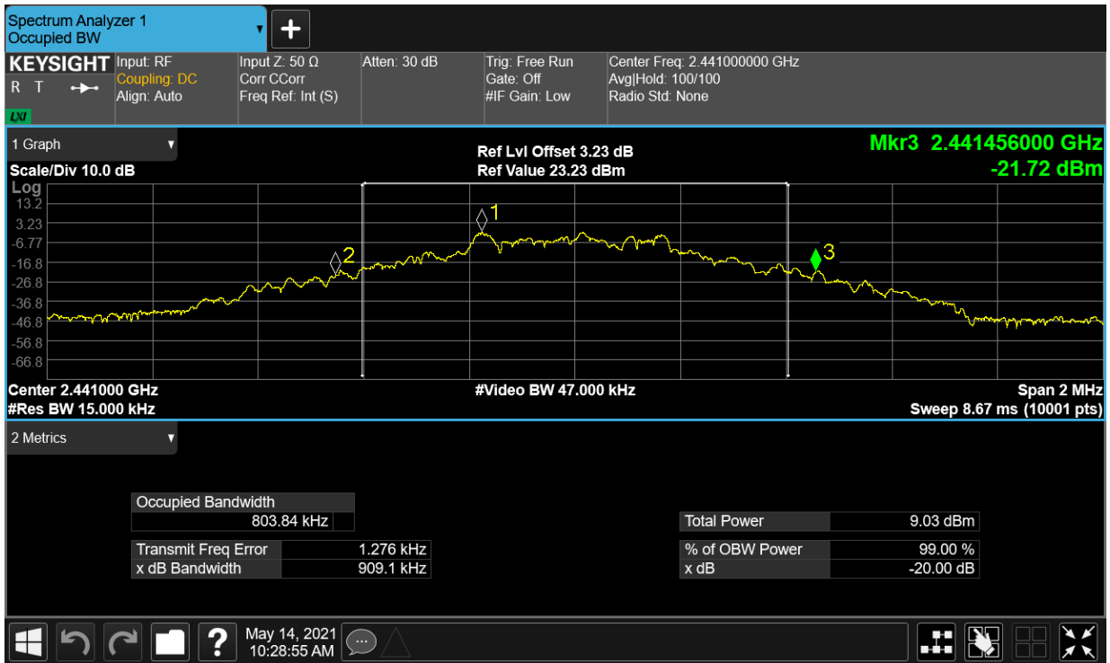
-20dB Bandwidth NVNT 1-DH1 2480MHz Ant1
