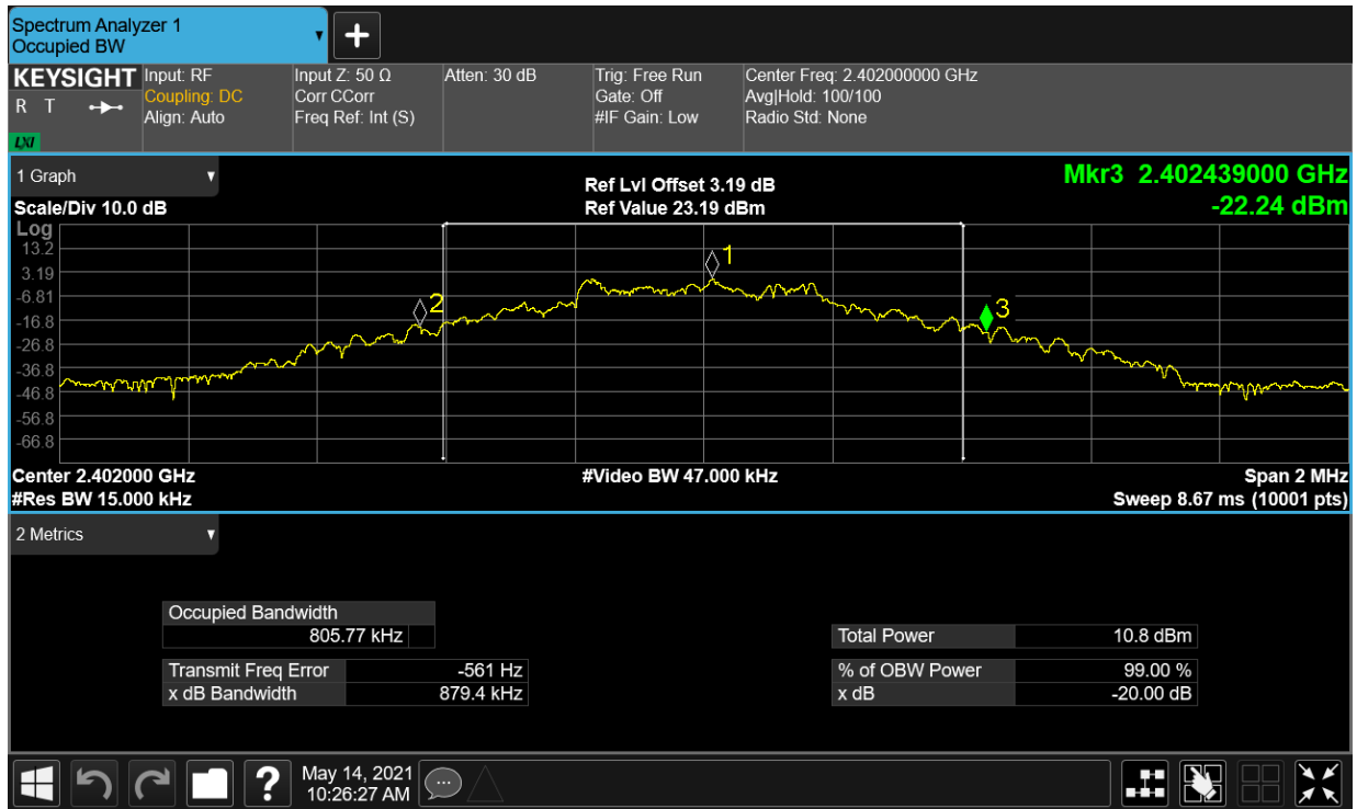
-20dB Bandwidth NVNT 1-DH1 2441MHz Ant1
