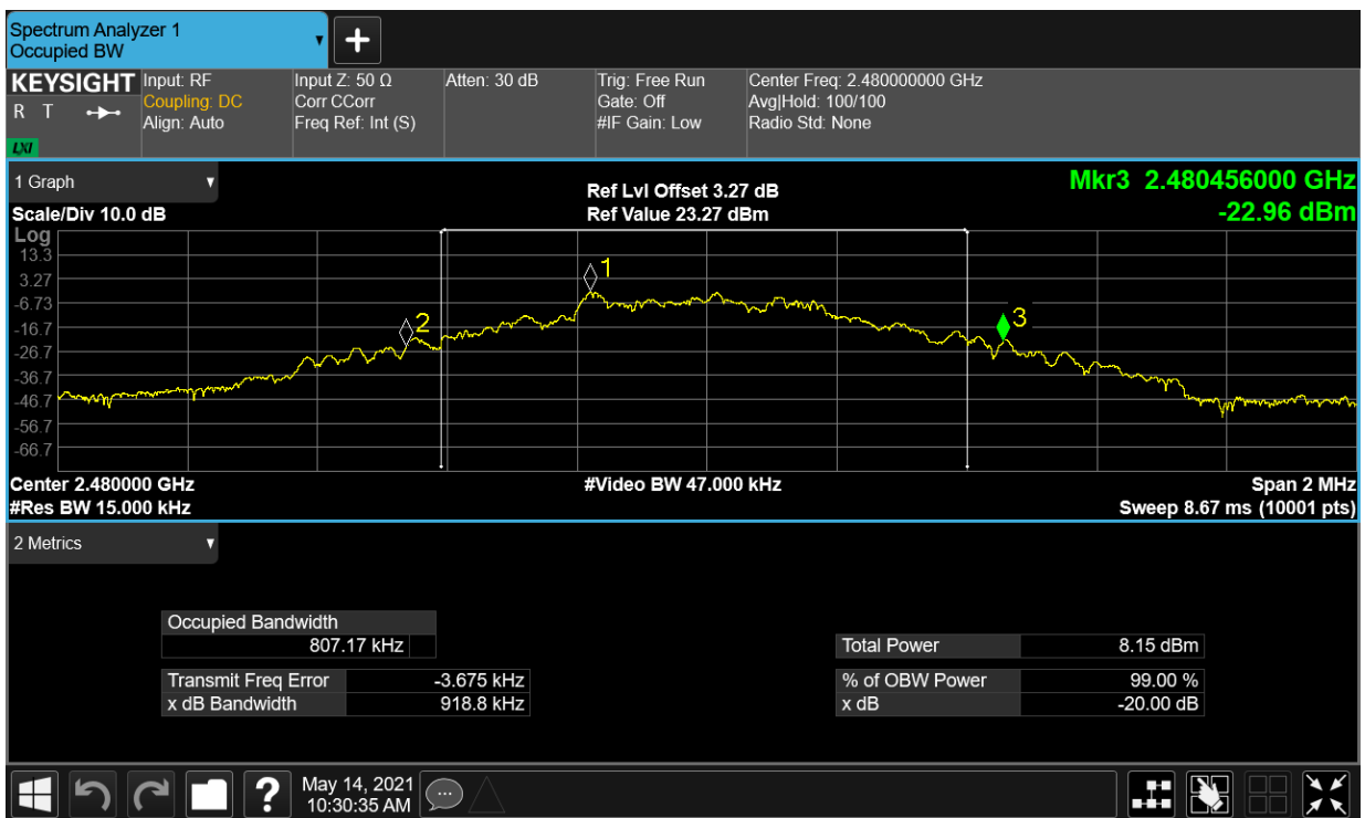
-20dB Bandwidth NVNT 2-DH1 2402MHz Ant1
