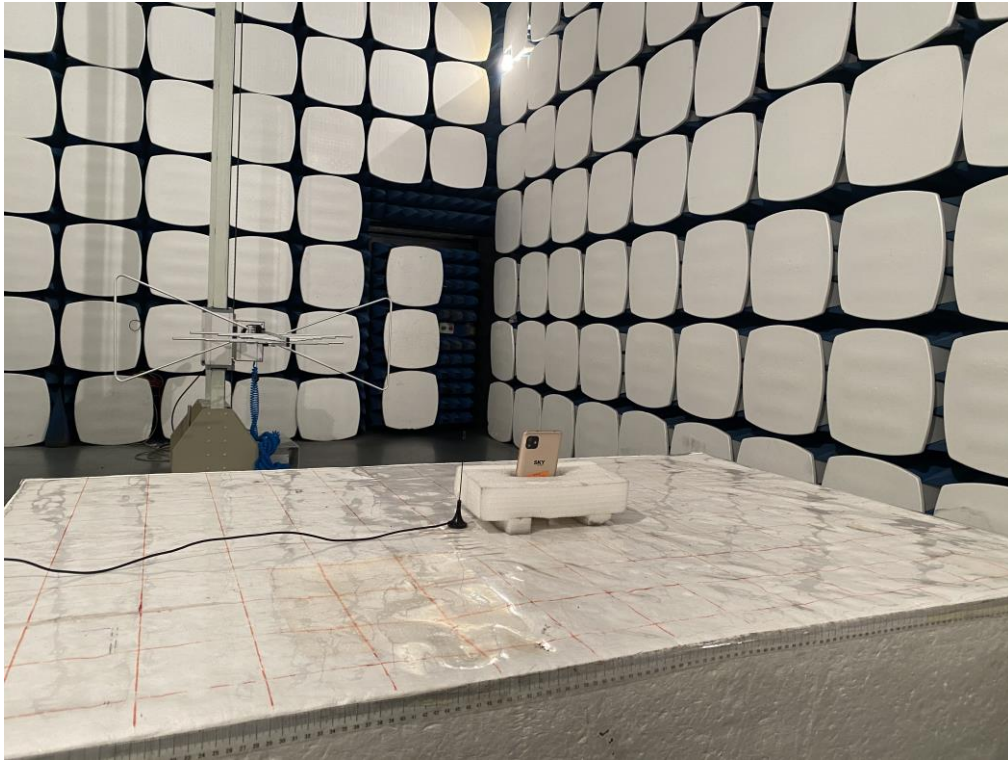
Radiated Spurious Emission Below 1GHz
