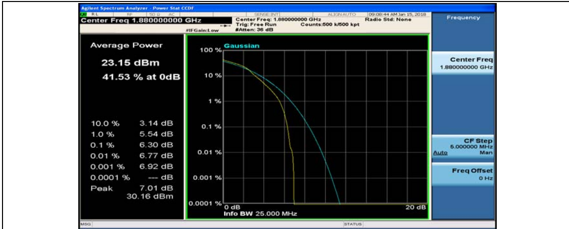
(Channel Bandwidth: 5 MHz)_MCH_16QAM_12RB#0
