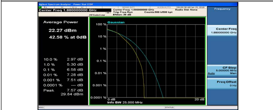
(Channel Bandwidth: 5 MHz)_MCH_16QAM_25RB#0
