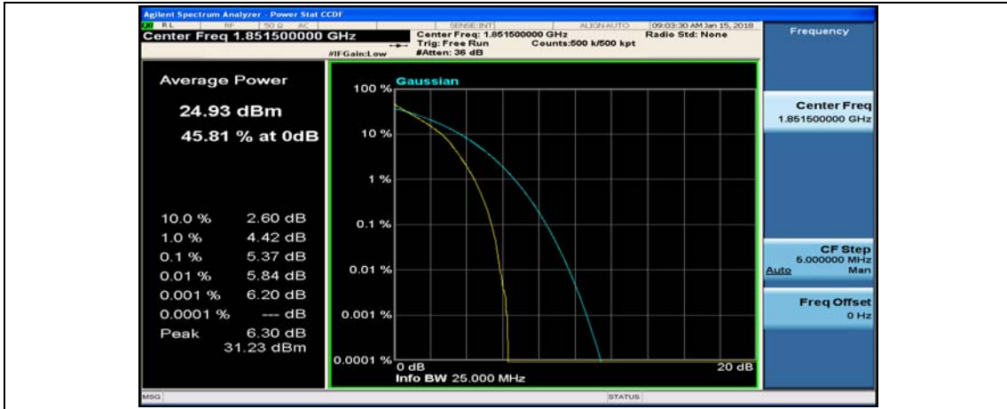
(Channel Bandwidth: 3 MHz)_MCH_QPSK_1RB#0
