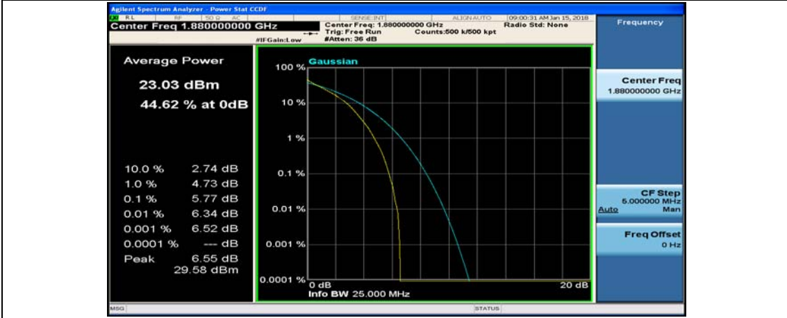
(Channel Bandwidth: 1.4 MHz)_MCH_QPSK_6RB#0
