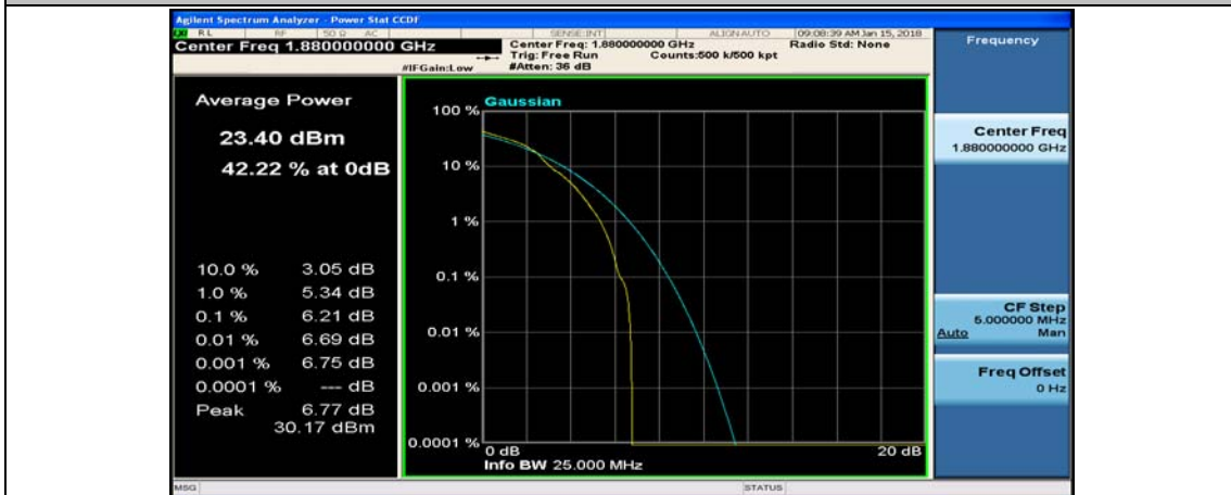
(Channel Bandwidth: 5 MHz)_MCH_16QAM_1RB#24
