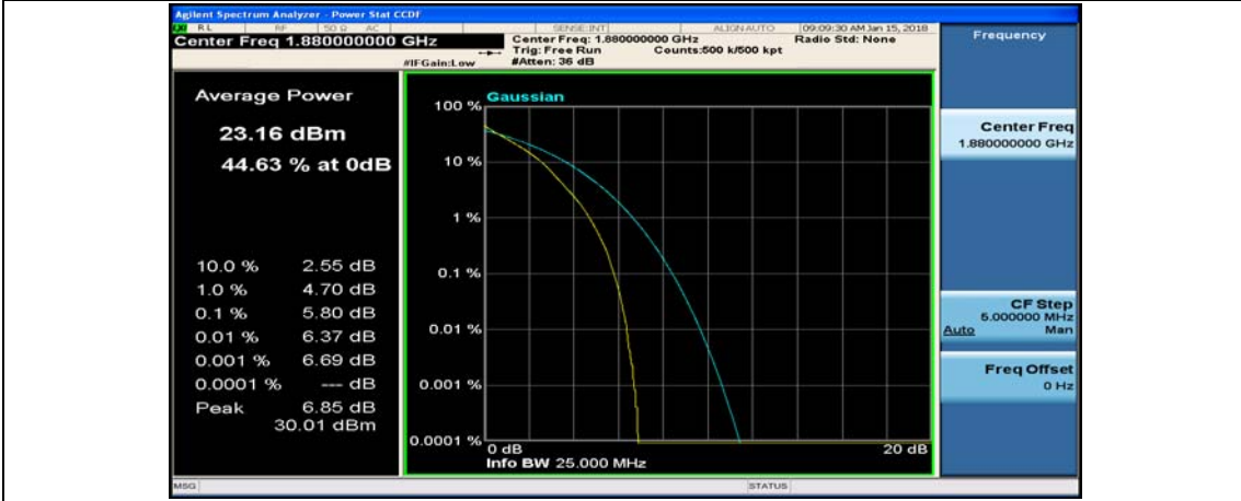
(Channel Bandwidth: 5 MHz)_MCH_QPSK_25RB#0
