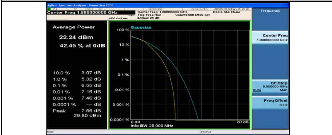
(Channel Bandwidth: 3 MHz)_MCH_16QAM_15RB#0
