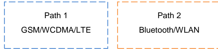
Fig.15.1 Simultaneous Transmission Paths
