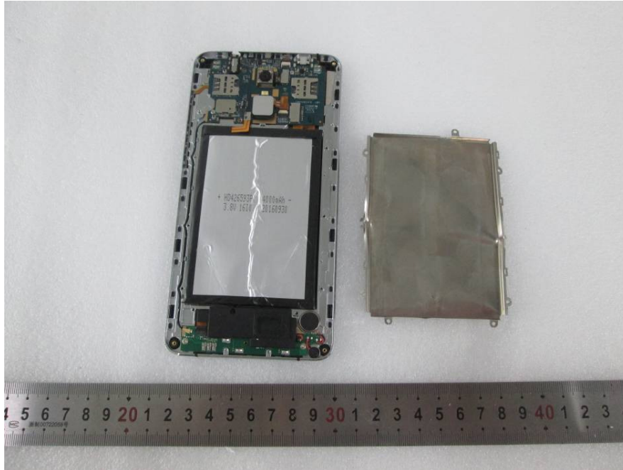
EUT – Cover off View 3
