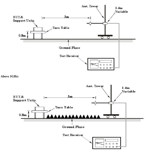
The radiated emission tests were performed in the 3 meters chamber test site, using the setup accordance with the ANSI C63.4-2014. The specification used was the FCC Part 15.109 Class B limits.
