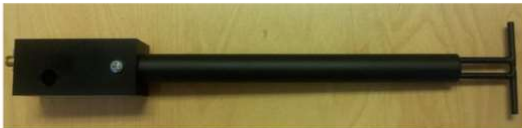
Figure 1 – MVG COMOSAR Validation Dipole
