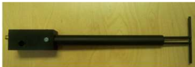
Figure 1 – MVG COMOSAR Validation Dipole
