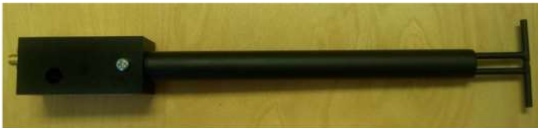
Figure 1 – MVG COMOSAR Validation Dipole
