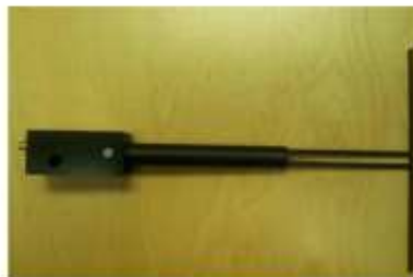
Figure 1 – MVG COMOSAR Validation Dipole
