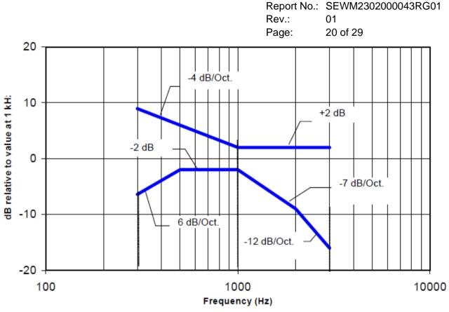
Figure 2 —Magnetic field frequency response for WDs with a field that exceeds -15dB(A/m) at 1 kHz
