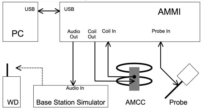
Fig. 2. T-coil signal measurement test setup
