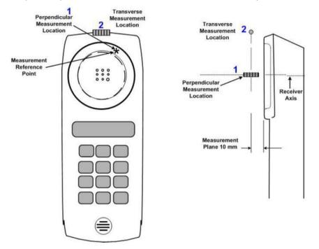
Figure 3 Axis and planes for WD audio frequency magnetic field measurements
