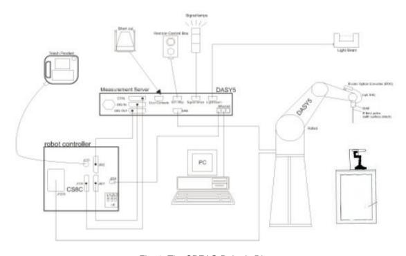
Fig. 1. The SPEAG Robotic Diagram
