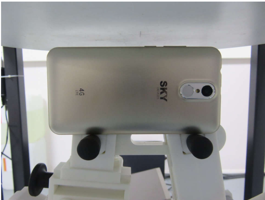
10mm body-worn Right Side Setup Photo (hotspot)
