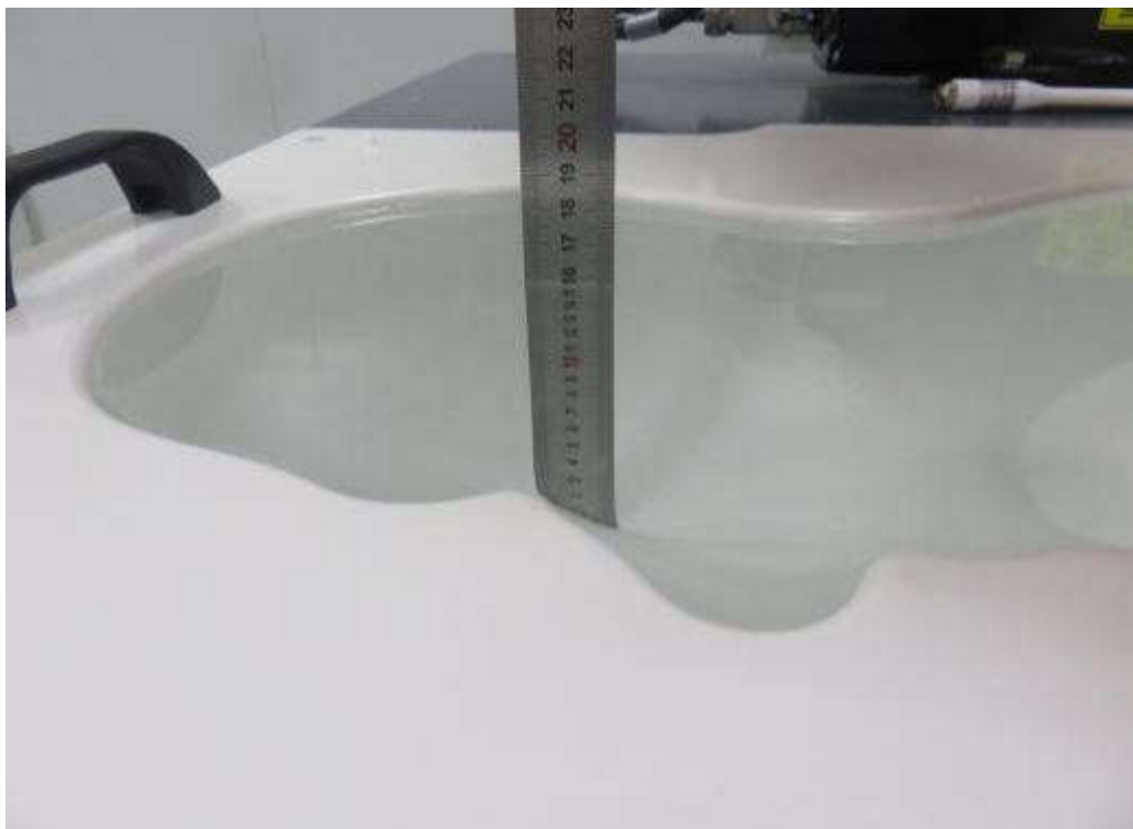
Photograph of the depth in the Head Phantom (1800MHz, 15.8cm depth)
