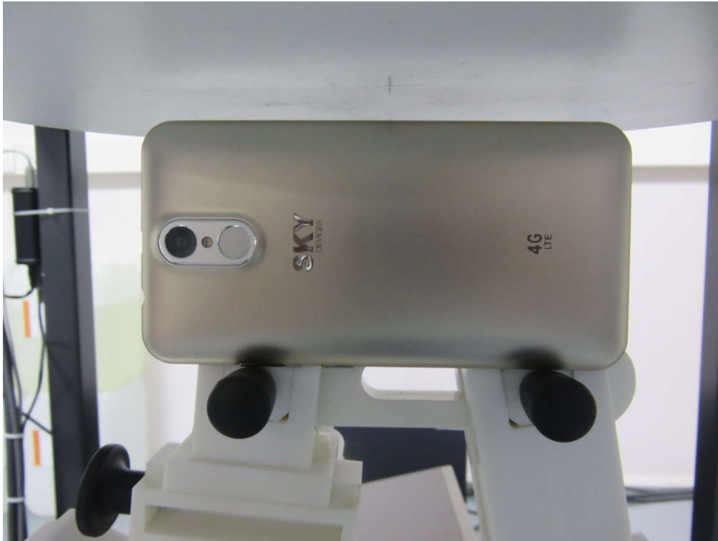
10mm body-worn Left Side Setup Photo(hotspot)
