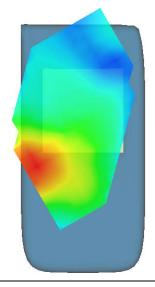
Test Mode: Hotspot GPRS1900MHz, High channel (Body FrontSide)
