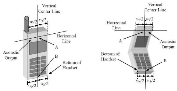
W<sub>t</sub>Width of the handset at the level of the acoustic
