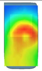
Test Mode:WCDMA Band V,Highchannel(Head RightCheek)
