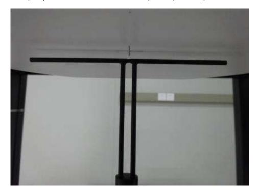
Photo of Dipole Setup
