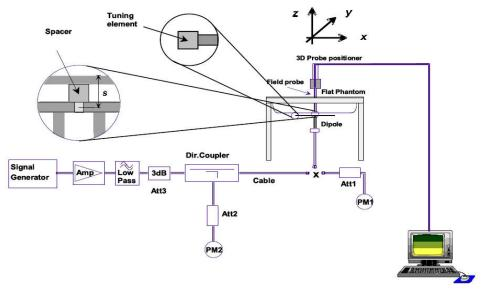
The output power on dipole port must be calibrated to 20 dBm (100mW) before dipole is connected.
