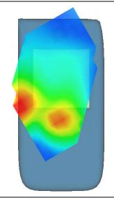
Test Mode: Hotspot WCDMA Band II, Middle channel (Body Front Side)
