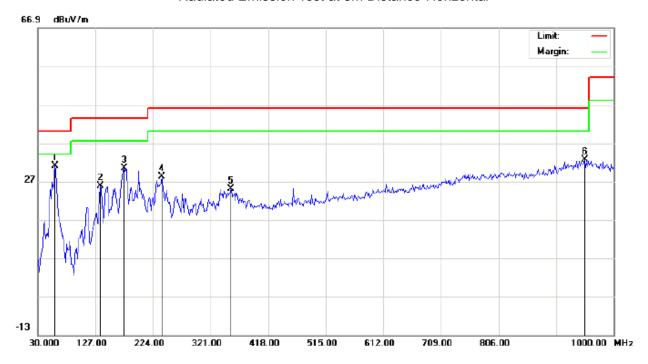
Site: site #1 Polarization: Horizontal Temperature: 22.8 Limit: FCC Class B 3M Radiation Power: AC 120V/60Hz Humidity: 56.1 %
