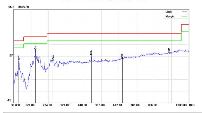
Site: site #1 Polarization: Vertical Temperature: 22.8 Limit: FCC Class B 3M Radiation Power: AC 120V/60Hz Humidity: 56.1 %
