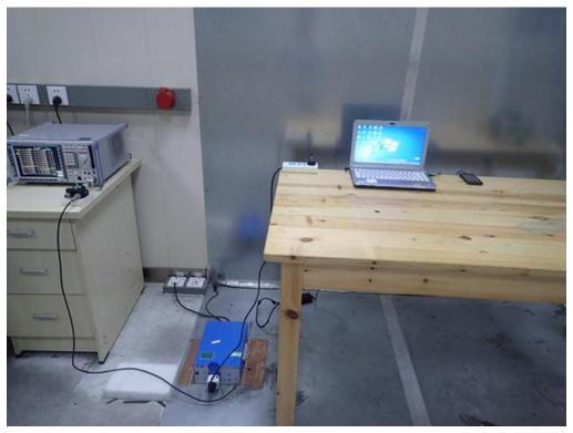
FCC RADIATED EMISSION TEST SETUP
