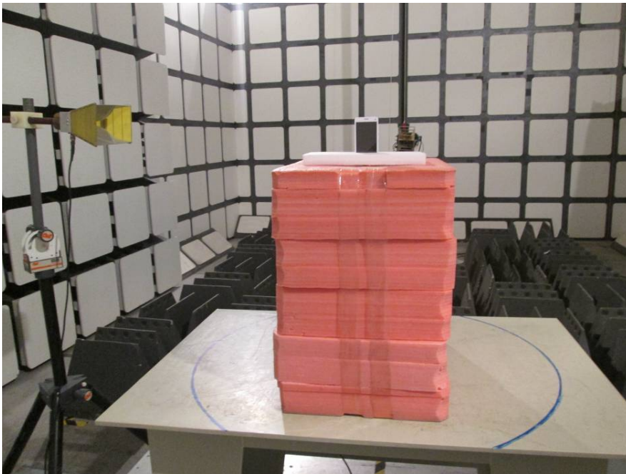
Radiated Emissions Test View (Above 1 GHz)
