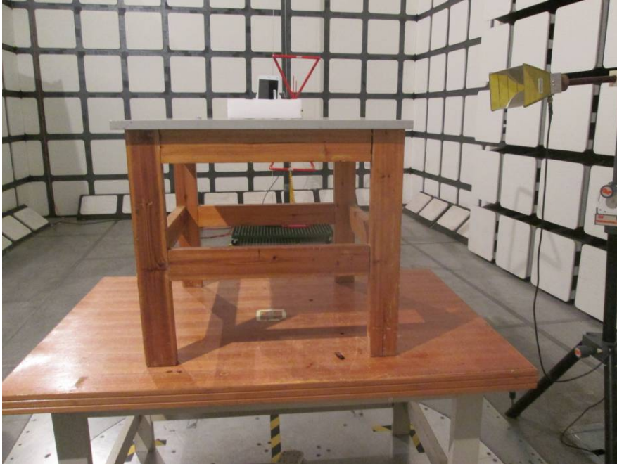
Radiated Emissions Test View (Below 1 GHz)
