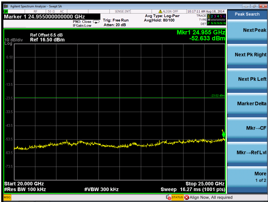
(Plot 6.6.2 B7: Channel 6: 2437MHz @ 802.11g)
