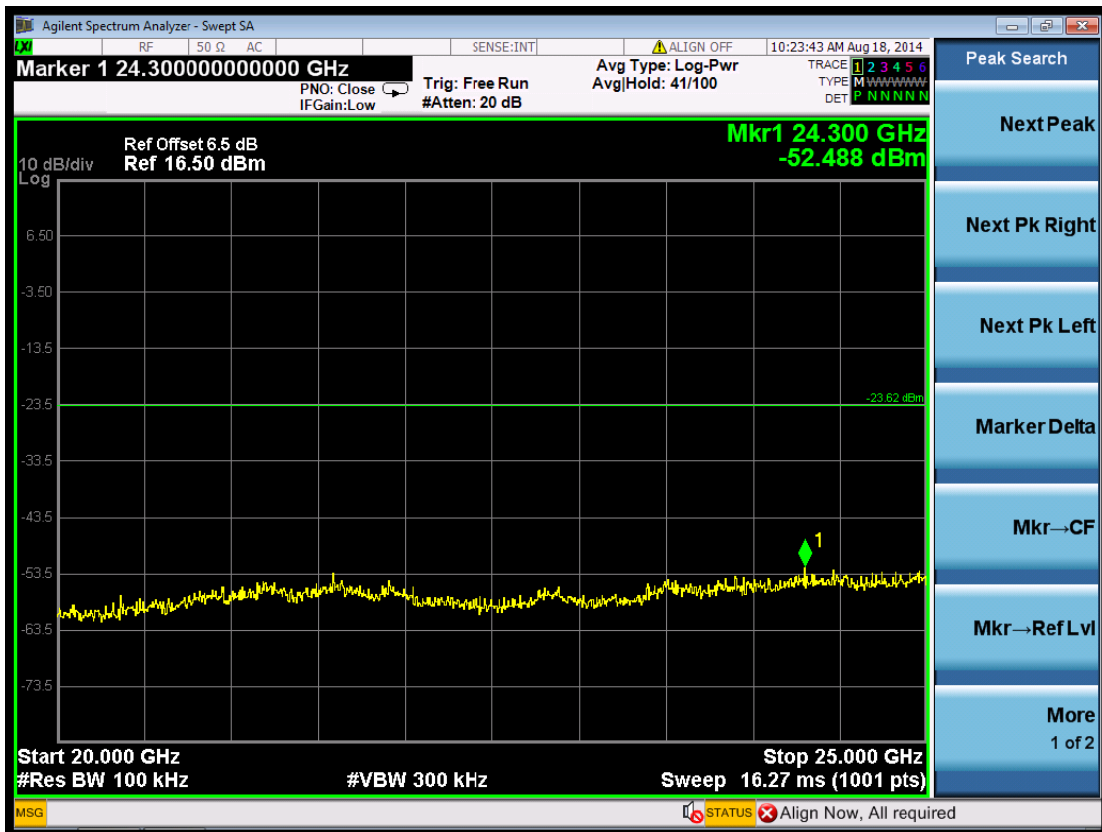
(Plot 6.6.3 A7: Channel 1: 2412MHz @ 802.11n HT20)
