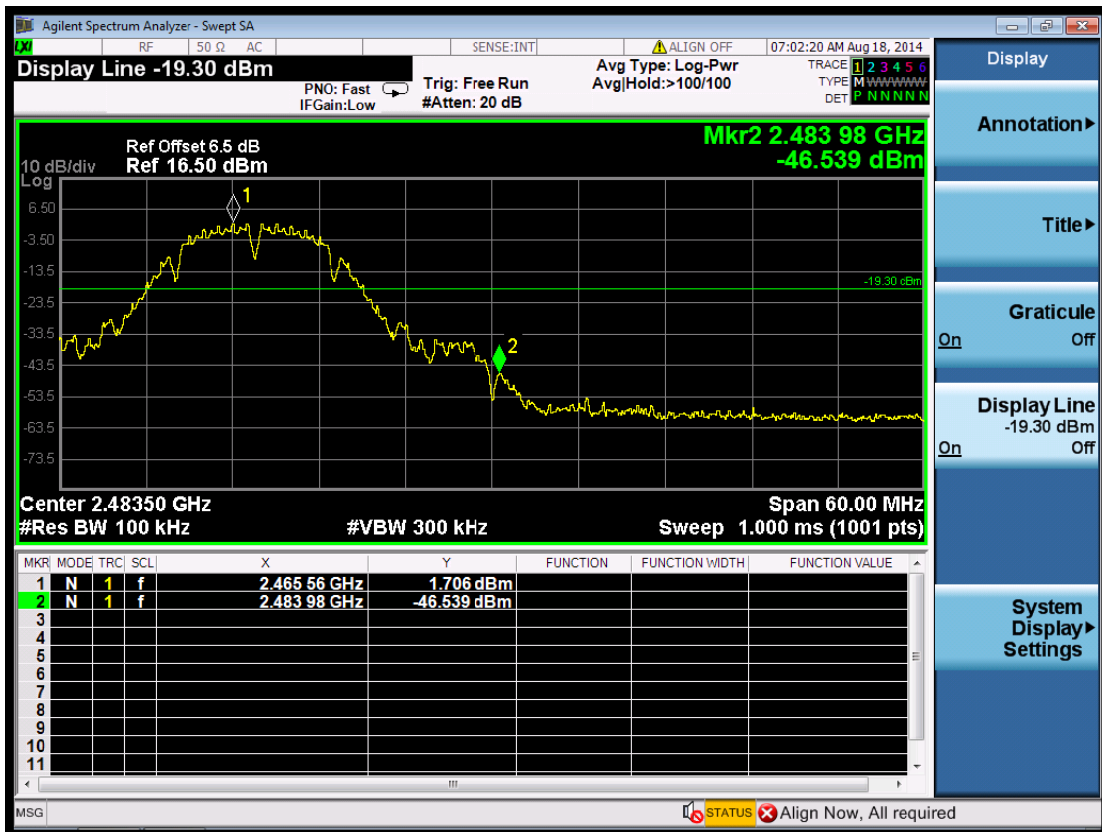
(Plot 6.6.1 E: Channel 11: 2462MHz @ 802.11b)
