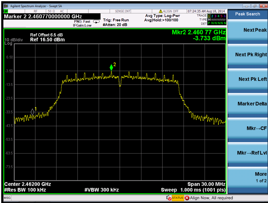
(Plot 6.6.2 C1: Channel 11: 2462MHz @ 802.11g)
