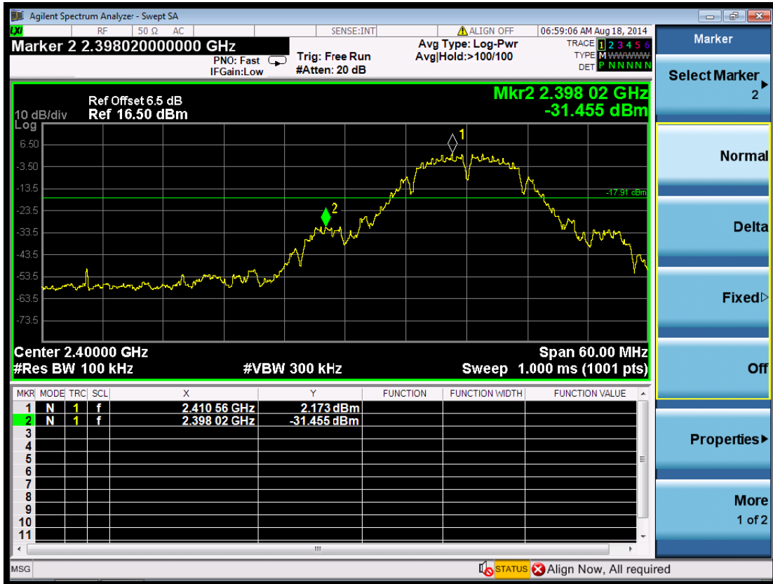
(Plot 6.6.1 D: Channel 1: 2412MHz @ 802.11b)
