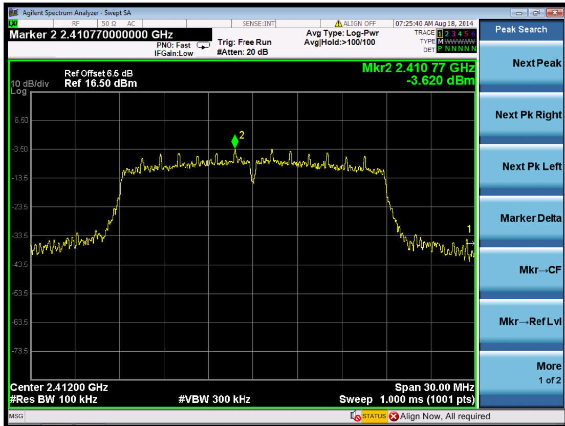
(Plot 6.6.3 A1: Channel 1: 2412MHz @ 802.11n HT20)
