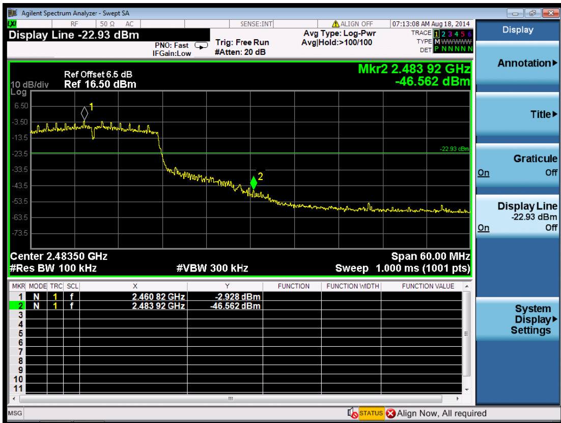
(Plot 6.6.3 E: Channel 11: 2462MHz @ 802.11n HT20)
