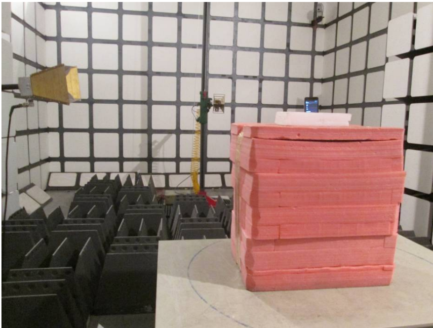
Radiated Emissions Test View (Above 1 GHz)
