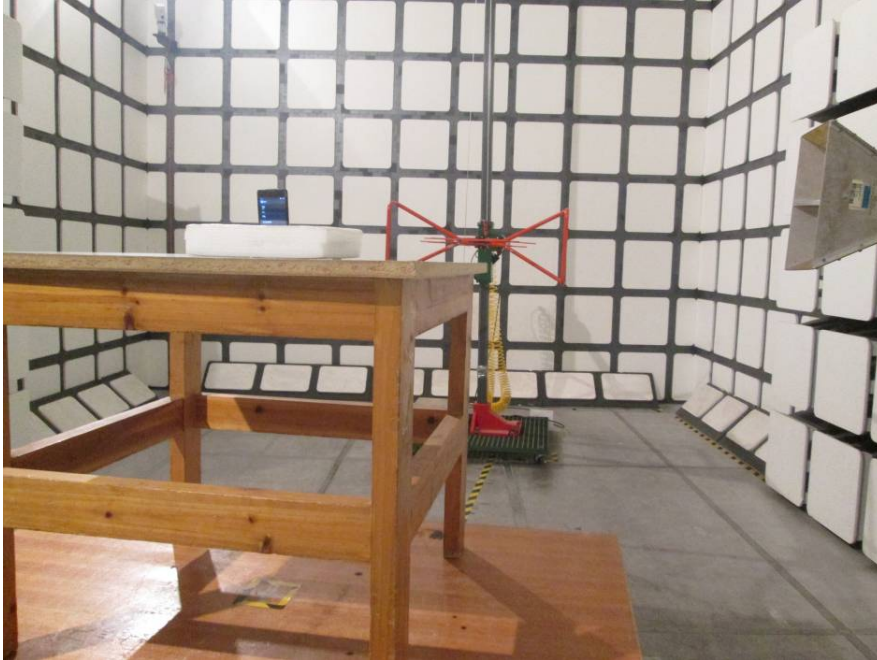
Radiated Emissions Test View (Below 1 GHz)
