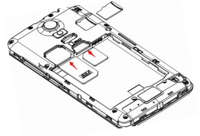
3) Slide the SIM card completely into the slot.
