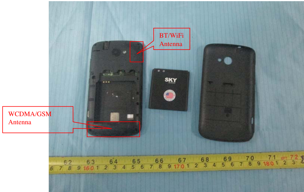
EUT – Cover off View 1
