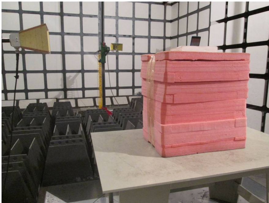
Radiated Emissions Test View (Above 1 GHz)
