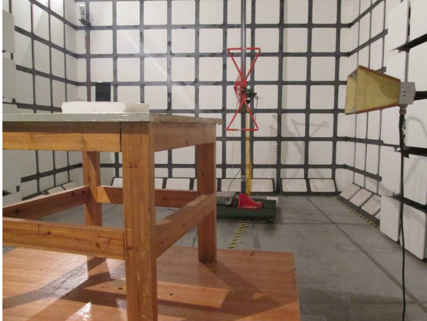
Radiated Emissions Test View (Below 1 GHz)
