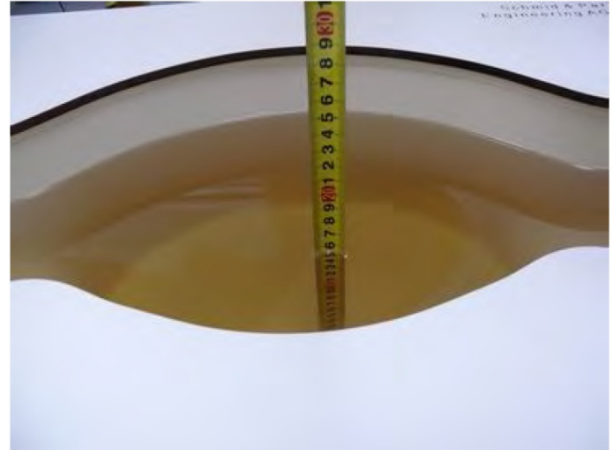
Liquid depth in the body phantom (835MHz)
