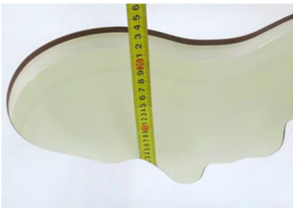
Liquid depth in the head phantom (835MHz)
