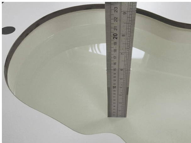
Liquid depth in the head phantom (2450MHz)
