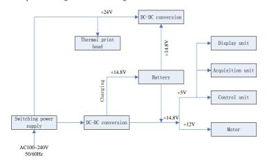
Figure4-1 Block diagram of power principle
