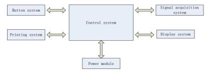
Figure 4-2 Block diagram of control unit
