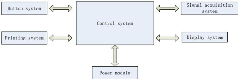
Figure 4-2 Block diagram of control unit
