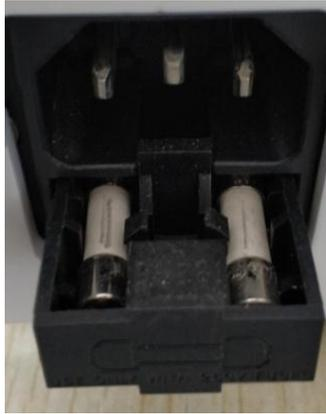
Figure 9-1 Replacing the fuse
