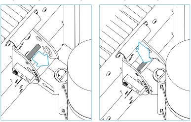
**Step 5.** Return outer hex/flange bolt to bracket, orient unit, and tighten. Do not torque the bolt at this time, as you may want to adjust the angle as part of link alignment. After alignment is complete, torque to 25 ft-lb (33 Nm).
