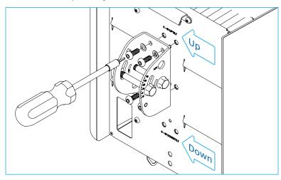
**Step 2.** Remove outer M8x70 hex/flange bolt from elevation-adjust bracket.
