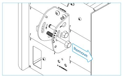
**Step 3.** Attach assembled gimbal and mounting bracket with groove opening in gimbal facing up. Do not torque the azimuth adjustment bolt at this time, as you may want to adjust the angle as part of link alignment. After alignment is complete, torque to 25 ft-lb (33 Nm).
