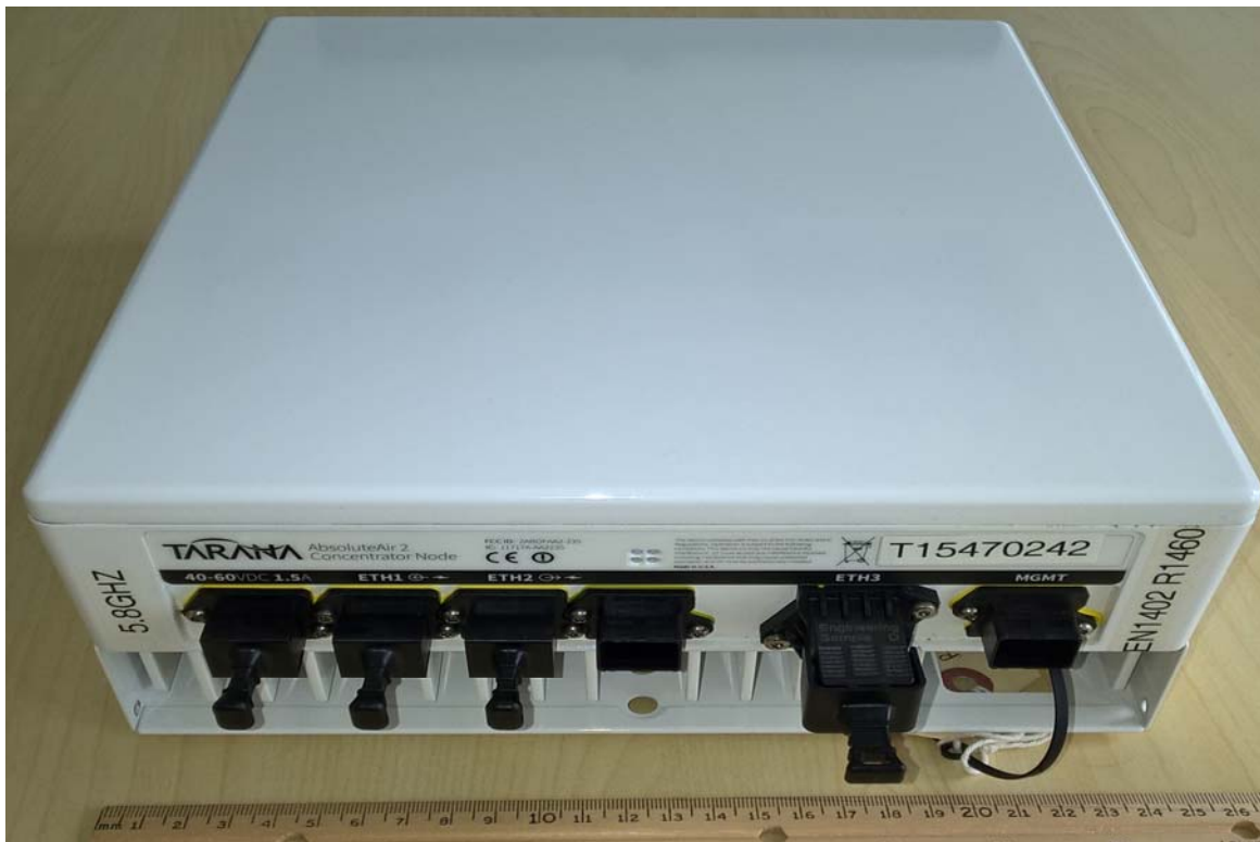
Photo 2- Top View SP Model with Connectors
