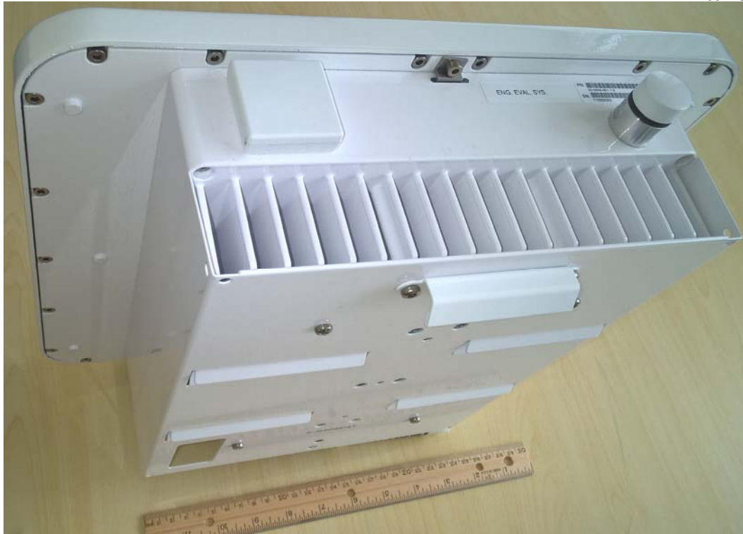
Photo 3- Back View with GPS & DFS Antennas (mounted on ALL Models) – FP Models
